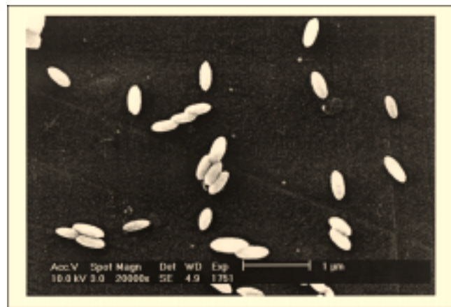
Figure 6. SEM micrograph of hematite particles.
